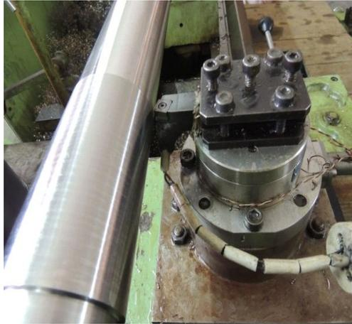
**Fig.1 Photograph of experimental setup for turning of 17-4 PH Stainless steel.**
